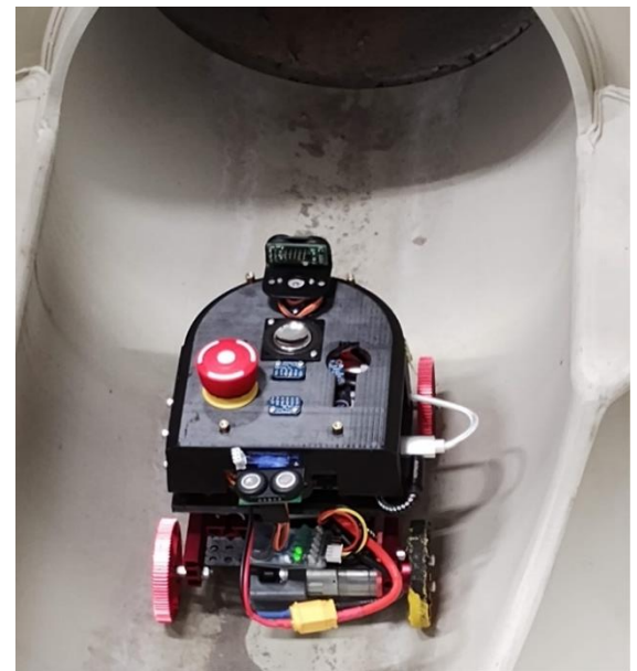
Figure SEQ Figure 1* ARABIC 1: Early prototype of the 'Tankbot' merging from a 300 mm diameter
