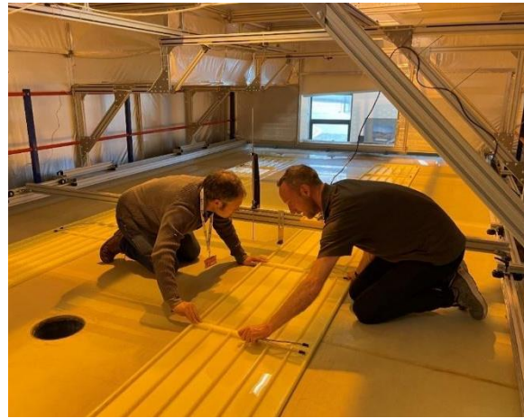
Setting up a model street to study contaminant spreading in urban flood waters, at the above-below ground flume at Sheffield University
